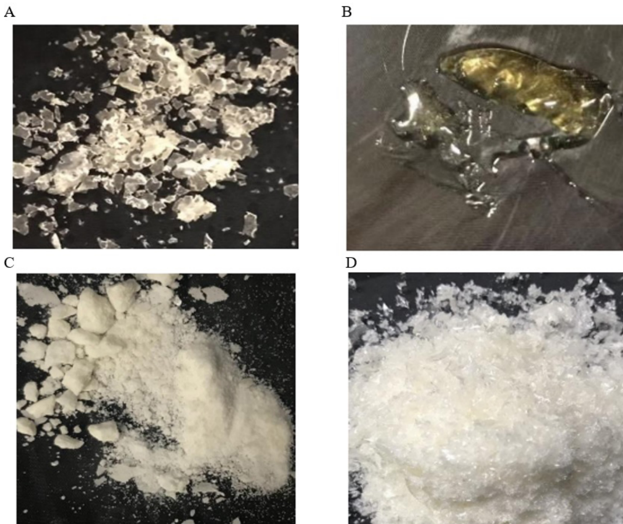
Fig. 4. Lactobionic acid samples were obtained through microbial fermentation using Pseudomonas taetrolens . After bioreactor fermentation, the product was centrifuged and microfiltered to remove bacteria, then subjected to further processing: (A) Dried at 40 °C in a thin layer. (B) Concentrated to 40% total solid content and dried at 40 °C. (C) Precipitated with 96% ethanol from the concentrated product (40% total solid content), followed by drying at 40 °C. (D) Freeze-dried from the concentrated product (40% total solid content) [68].
