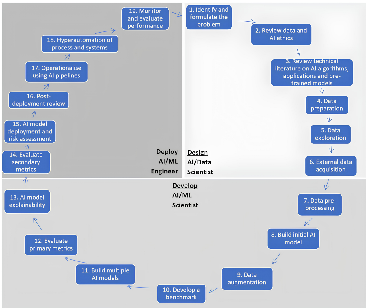
Fig. 8. CDAC AI life cycle. Reprinted from Silva and Alahakoon, 2022 , p. 6. CDAC, Centre for Data Analytics and Cognition AI life cycle. ML, Machine Learning.
