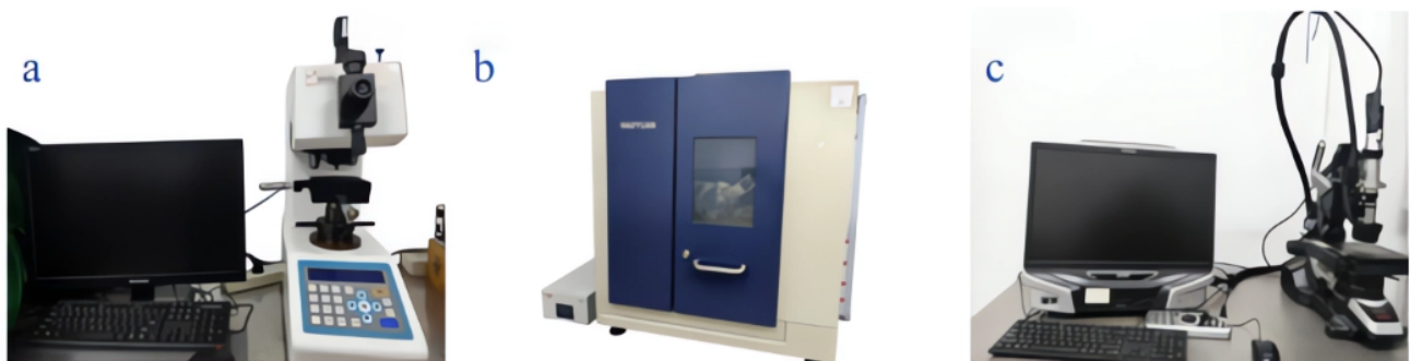
Fig. 3. Experimental instruments. (a) Huayin HV-1000A Vickers Optical Microhardness Tester. (b) DX-2700A X-ray Diffractometer. (c) Keyence VHX-5000 Super Depth of Field 3D Digital Microscope.
