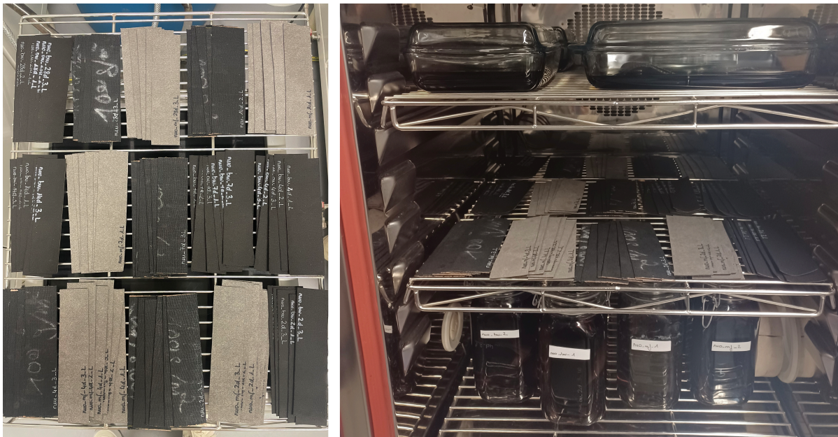
Fig. 4. Placement of the composite samples in the climate chamber: dry ageing on metal grids (left); dry and wet ageing in glass vessels (right).
