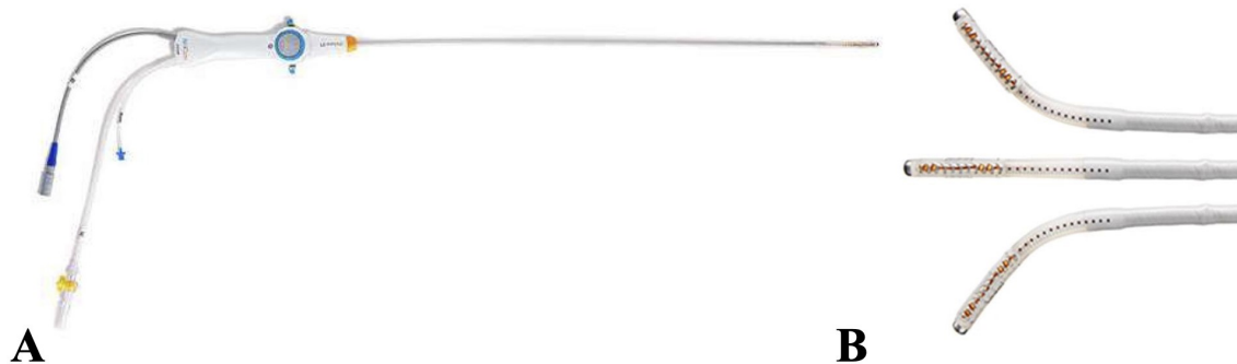
Fig. 3. The Epi-Sense™ epicardial ablation device. (A) Overview of the Epi-Sense™ device and delivery system. (B) Magnified image showing the helical RF coil and integrated suction channels that stabilize the probe during lesion creation. Reproduced with permission from AtriCure.
