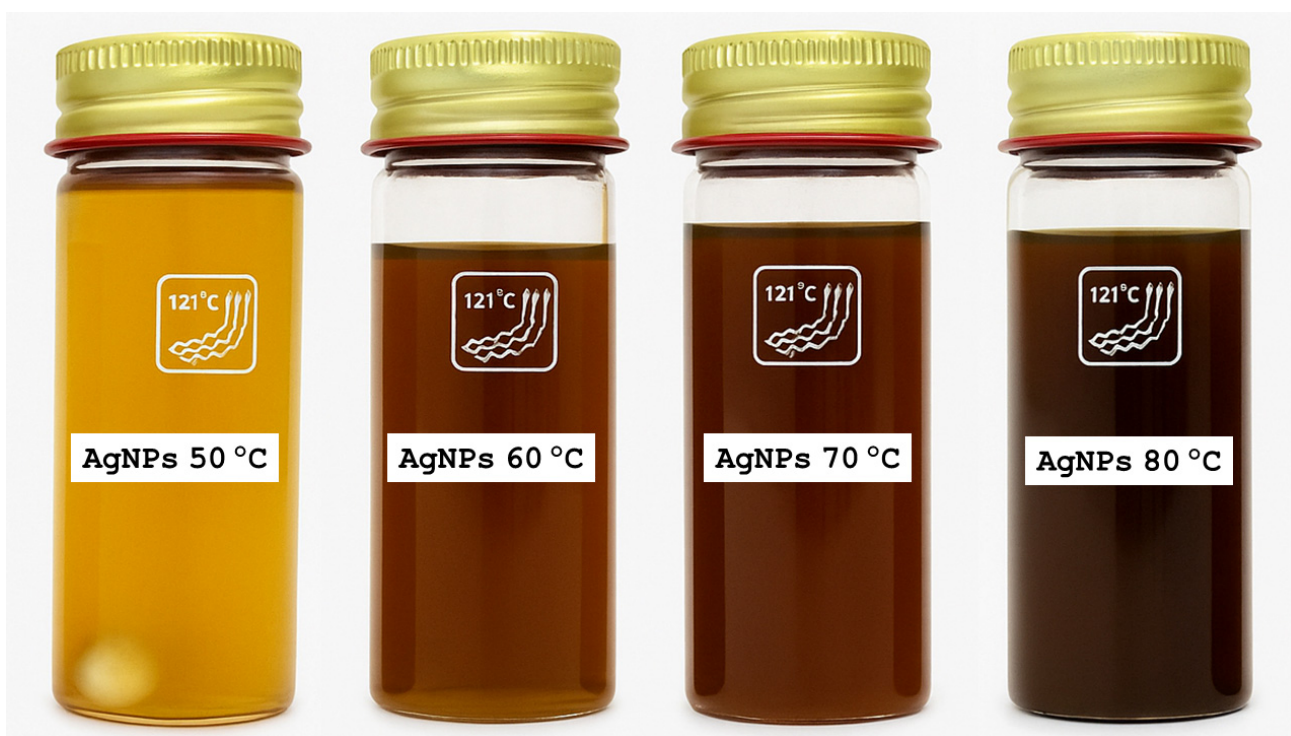
Fig. 2. Silver nanoparticle solution synthesized by the green method at, 50 °C, 60 °C, 70 °C, 80 °C.
