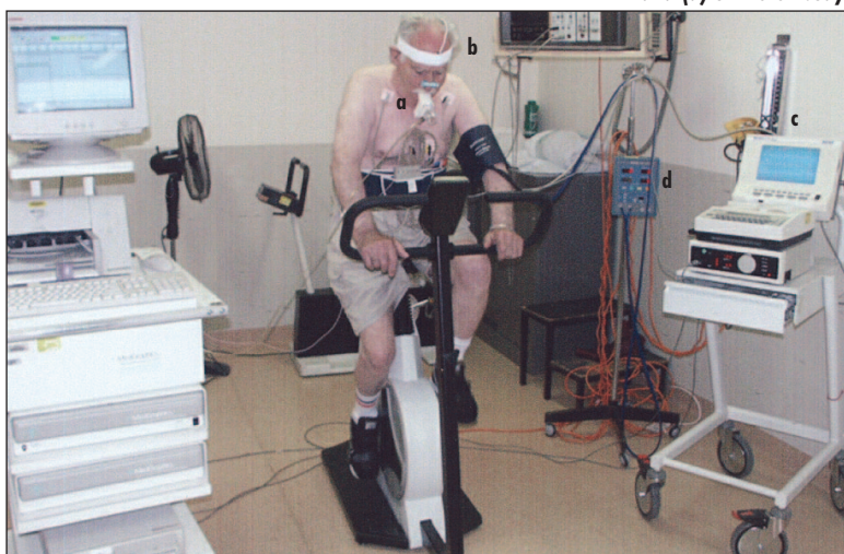
Figure 1. An elderly patient cycling a bicycle ergometer. Note (a) the small and lightweight mouthpiece, (b) the oximeter probe attached to the forehead, (c) the electrocardiograph and (d) oximeter body.
