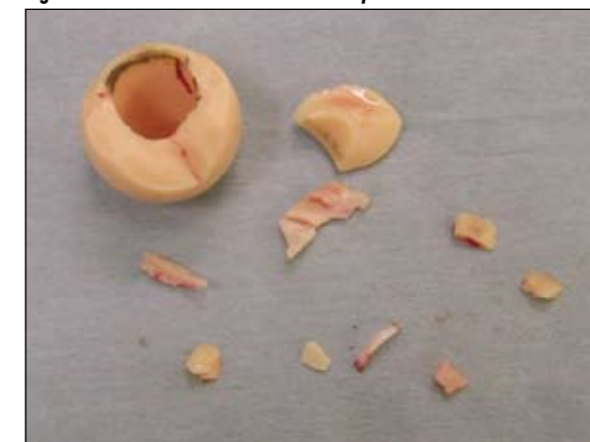
Figure 4. Fracture of brittle ceramic component.
