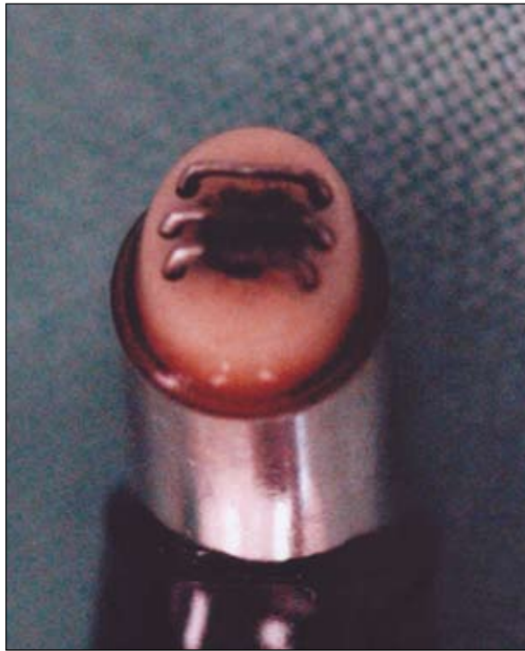
Figure 1. Coblation wand tip electrodes.
