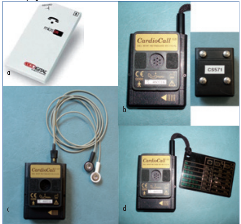
Figure 6. The electrocardiogram event is recorded by holding the recorder on the chest and pressing a 'record button'. The patient then transmits the electrocardiogram down a standard telephone line to a receiving centre.
