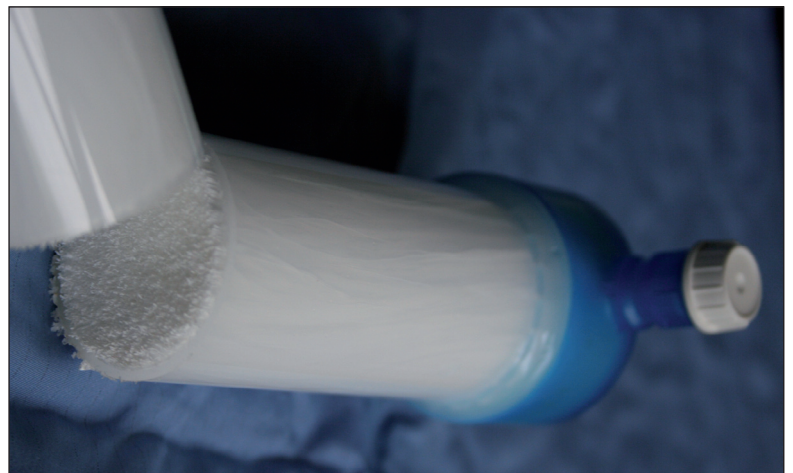
Figure 2. Hollow-fibre device shown in cross-section. Each of the thousands of hollow-fibres bundled into the device comprise a wall of a semi-permeable material and a lumen through which blood flows – collectively, the ‘blood compartment’. In diffusive modalities, dialysate flows around the outside of the hollow fibres in the ‘dialysate compartment’. Flow of this solution, constituted to restore physiological plasma solute concentrations, is usually in an opposite – or counter-current – fashion to blood to enhance concentration gradients. In purely convective modalities there is no dialysate flow. The dialysate compartment provides the space where ultrafiltrate initially accumulates after first being drawn across the membrane. Membrane properties dictate whether use is predominantly convective or diffusive.
