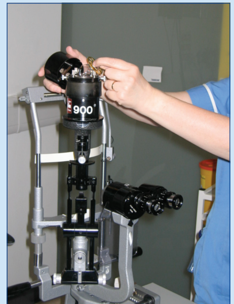
Figure 25. Changing the light bulb. Ensure the power is disconnected.
