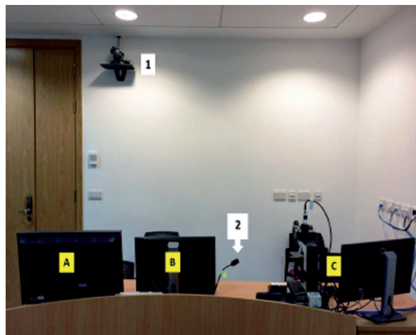
Figure 3. Typical radiology, multidisciplinary team coordinator and pathology setup for a videoconferencing multidisciplinary team meeting. A. Workstation for radiologist. B. Computer for multidisciplinary team coordinator. C. Microscope and PC for pathologist. 1. A wall-mounted camera with a 65–75° field of view. 2. Microphone.
