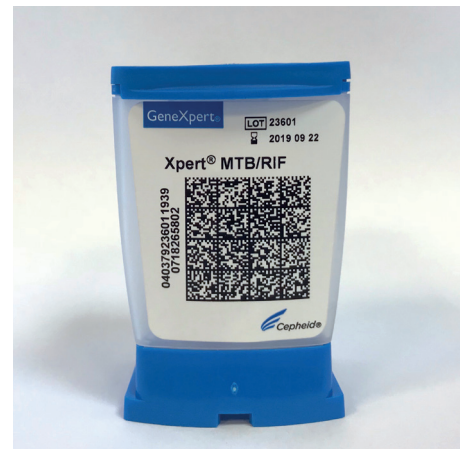
Figure 3. The GeneXpert cartridge for tuberculosis polymerase chain reaction testing.
