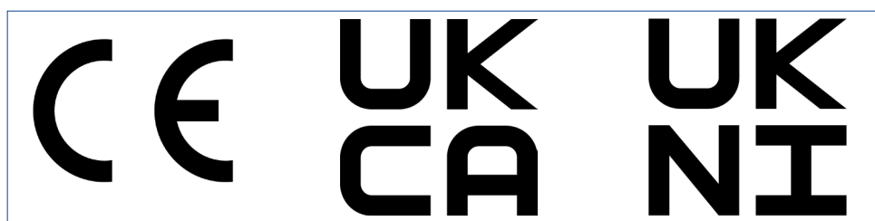
Figure 1. Official notation for the CE mark, the UK Conformity Assessment mark and the UKNI mark.
