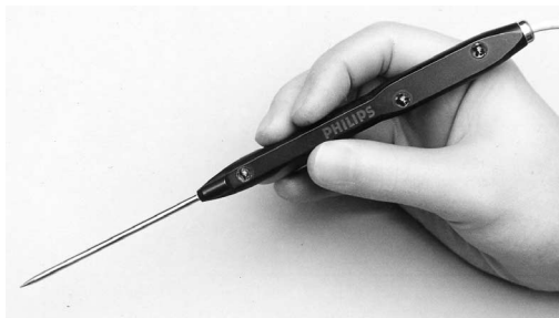
Figure 5. Infra-red optically tracked surgical 'pointer'. The pointer is held by the surgeon and its exact position calculated by the neuronavigation system by the detection of flashes from the three infra-red light-emitting diodes by a three-dimensional camera array.
