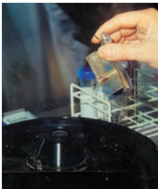
Figure 1. Cytospin chambers are loaded in the cytospin head which is placed within a biosafety cabinet.
