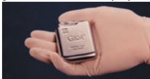
Figure 3. Typical implantable defibrillator generator.
