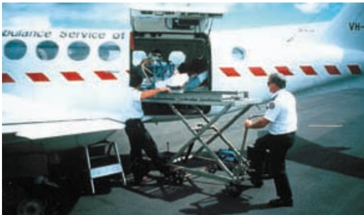
Figure 4. Dedicated fixed-wing aircraft showing cargo door adapted for stretcher access.
