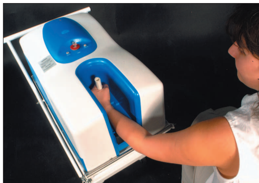
Figure 2. A peripheral dual X-ray absorptiometry (DXA) scanner for measuring forearm bone mineral density. Peripheral DXA systems are smaller and cheaper than spine and hip systems such as that shown in Figure 1.
