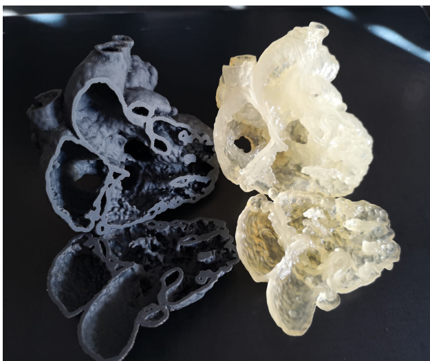
Fig. 2. Two sets of heart models that feature different types of CHD (double outlet right ventricle is shown in this image) were printed in two different printing materials, Flexible V4 Resin from Formlabs (left), and TPU80A from Fabbxible Technology (right). Reprint with permission under the open access from Lau et al. [15].
