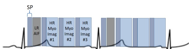
Fig. 24. Scheme of a dual-sequence for QP. A low-resolution (LR) AIF sequence precedes the set of slices of a high-resolution (HR) sequence for myocardial perfusion imaging. Each image has a saturation recovery preparation (SP).
